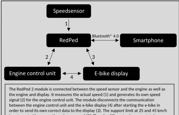
is outsmarted by generating a lower speed (2). Thereby different values, e.g. total distance calculated incorrectly by the engine control unit, but corrected by the RedPed 2 module (3) as long as it is connected.
