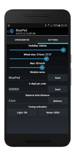
**Visibility:** Can be set to values between 0 and 240 seconds or "infinite". If visibility is set to 0, the app will no longer be able to find the module after disconnecting or restarting the E-Bike.
