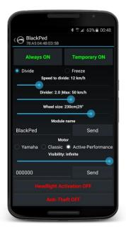
**Speed to freeze:** If the speed reaches this value, it will freeze. Minimum value is 10 km/h.
