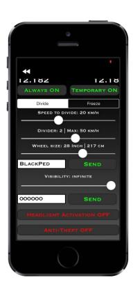
**PIN:** Consists of exactly 6 digits. If too few digits are entered, the value will be fillled with zeros. (1 = 000001; 345 = 000345)
